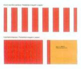
Mobile racking systems do not need aisles at all. Thus provides the highest room exploitation. Operated by radio control or by pushing a button, the racking system opens at the place where you want to access your goods. Cantilever racking can also be transformed into a mobile racking.
