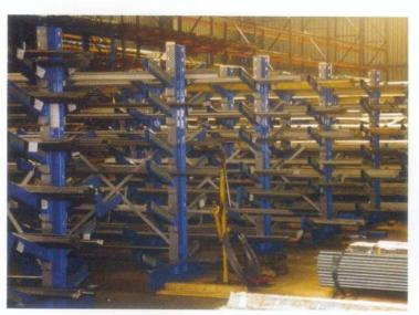
Racking with inclinable arms are serviced by overhead crane. Invariably, long material will be manually handled. We can supply this range with: Load protection
