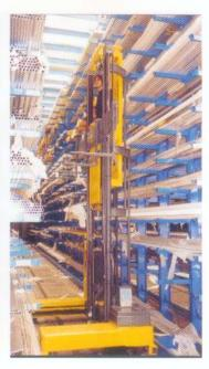
The OHRA Cantilever product range for the steel and metal trade involves "light" racking for the storage of aluminium and tube material, and "heavy" racking for solid material, heavy sheet metal and coils with a single weight of up to 15 tons. With different solutions we adapt the racking technology according to the individual flow (e.g. coils in standing, flat or hanging position) and the corresponding transport
